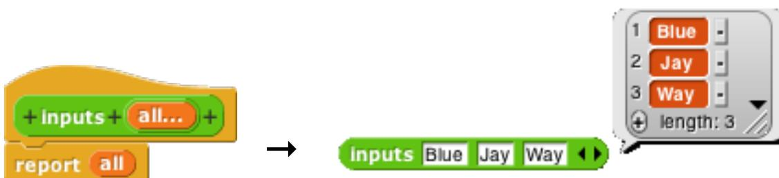
The ellipsis (...) in the orange input slot name box in the prototype indicates a Multiple input.
